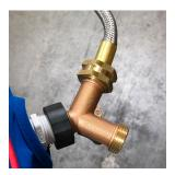
2. Attach other Y Valve to the output side of the system (right side when facing).
